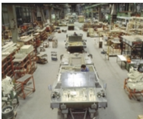
ELVO • Light armoured vehicle "Leonidas" assembly line
